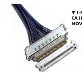
Board-to-Board FPC Connector (accepts FPC [flexible printed circuit] on the plug connector and rigid PCB on the receptacle connector) have added shielding that eliminates the unwanted, radiated noise.
