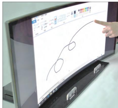
▲ Liyitec's 34-inch R1900 curved touch panel, the ultimate HMI solution for high-end curved monitor.
