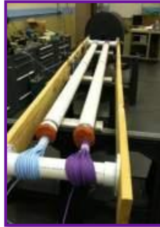
Conduit w/ Sealed Ends
