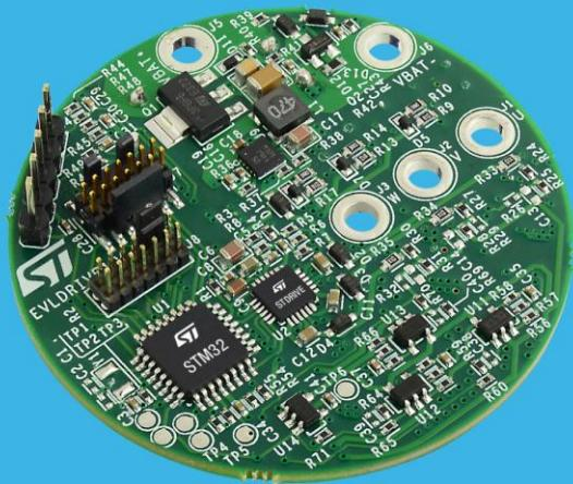
Tiny 750W motor-drive reference design
