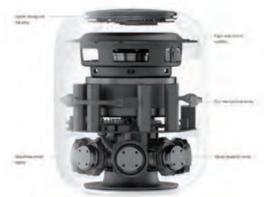
The interior of Apple HomePod Source: Company
