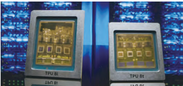
Google's 8th-generation TPU features a dual-chip architecture for the first time. (Google Cloud)
